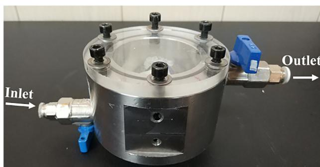
Fig. 1. Homemade Stainless steel gas chamber with gas inlet and outlet as well as a top glass window.
